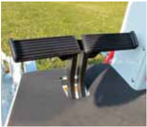
SERVICE BRAKES with separate pedal operation.
