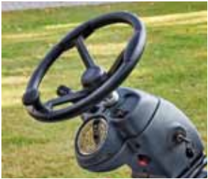
LIMITED TURNING RADIUS and steering wheel with hydro-guide operating on the rear wheels posteriori.
