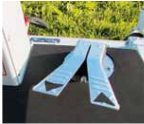
HYDROSTATIC TRANSMISSION with double pedal (forward/reverse) and two forward speed ranges.
