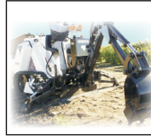
Backhoe Attach to regular bracket. Two models: one digs to 6'6" with 9' reach the other 8'6" with 11' reach. 12" buckets. Joystick control.
