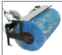
Rotary Broom - Hydraulically driven, 48" wide, 24" diameter, 30 degree left of right angling, steel and poly bristles.
