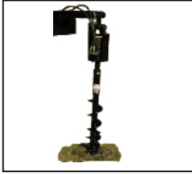
Post Hole Augers Direct drive head with 6,800 lb/in torque (peak) up to 105 RPM. Bits in 6, 9 and 12 inches. Also planetary heads.
