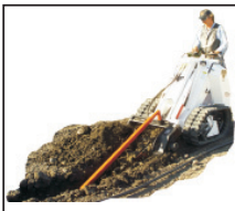
Trenchers - Hydraulic drive unit cuts up to 36" deep, in 4" or 6" widths. Optional 4" crumbler to clean debris from trench available.
