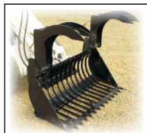
Grapple with Tines - loose materials drop through - two independent hydraulically controlled grapples.
