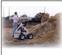
Hay and Manure Fork with Grapple - Four strong grapple tines with forks (or bucket) handle various materials. Hydraulically operated.
