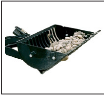
Grated Bucket separates rubble and stones from sand or earth. 43 in. wide with 2.5 in. tooth spacing and removable dirt plate.
