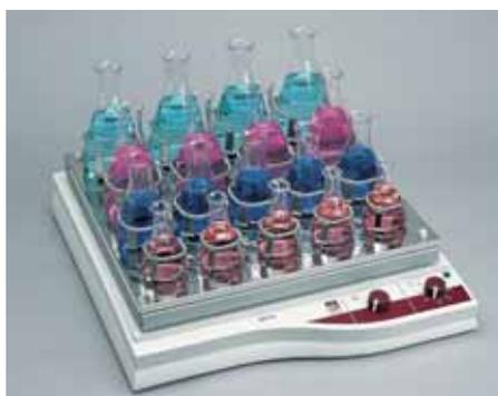
**3015** Analogue Orbital Shaker with Tray 3966 and Clamps for Erlenmeyer flasks 3983 - 3990
