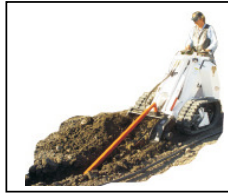
Trencher - 24" Cutting Depth 4" to 6" Chain Widths
