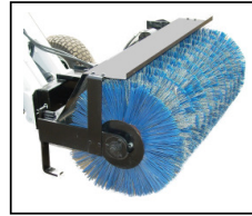
Brooms - 24" Dia x 36" Wide Angles - Steel & Poly Bristles
