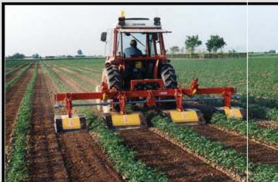
Multi-row rototiller mod. MSn/4(2SL+2L) working in tomatoes with hydraulic folding frame
