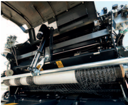
New dependable PowerBind net wrap system.
