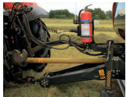
Height adjustable drawbar.
