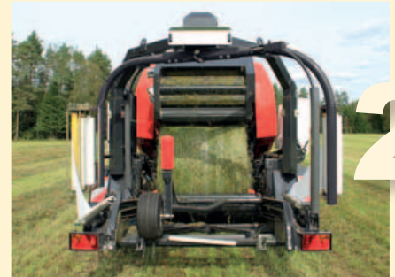
The bale is dropped directly onto the wrapping table.
