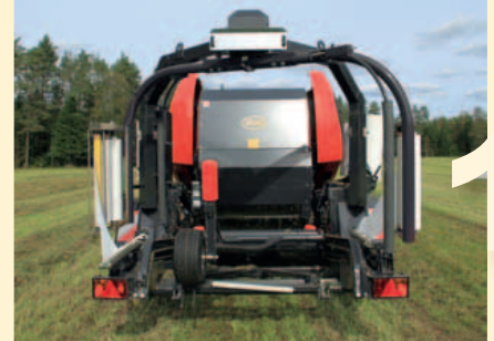
Once the net is applied to the bale the wrapping table is transferred to the tailgate of the baler.
