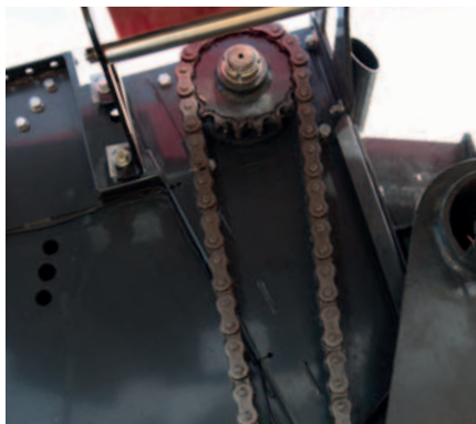
Main bale chamber drive is by heavy duty 1 1/4" pitch chain for longer lifetime and reduced maintenance.
