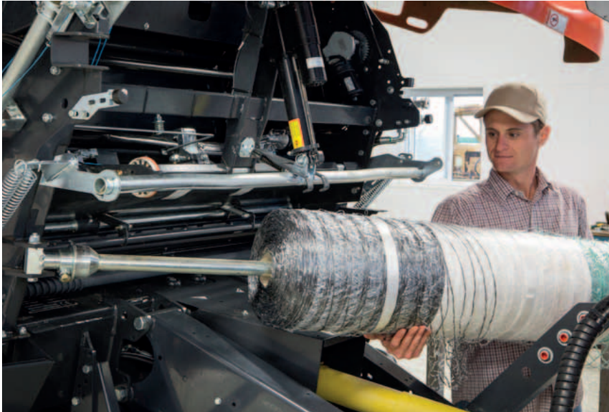
The very low loading height and the very easy threading of the system mean minimum downtime and maximum time baling.
