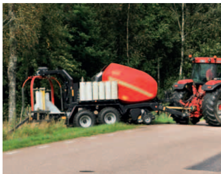
The tandem axle provides good stability.
