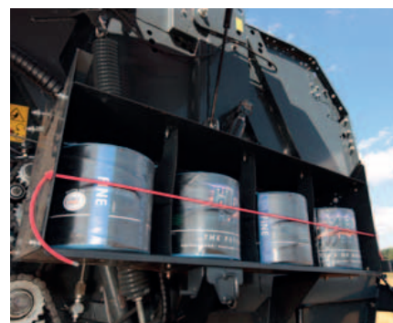
Convenient easy access storage for net and twine for long working days.
