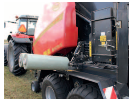
The extra stretch films are lowered hydraulically for easy change.
