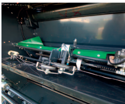
Twin tube fast operating twine binding system.
