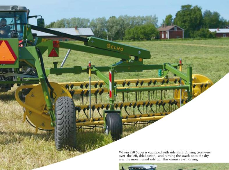
Thanks to the throwing movement of the tines of the V-Twin swather, the risk of stones in the swaths will be reduced, which can present a problem with the traditional swathers that roll on the ground. This also reduces the risk of breakage for the harvester following the swather.
