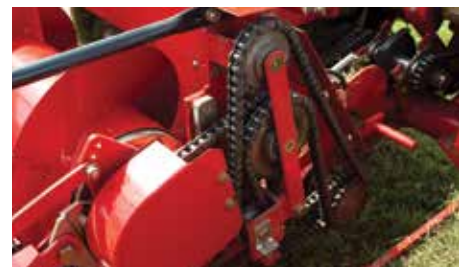
All gears and chains are hardened which gives a considerably longer life.
