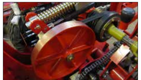
Reverse system is activated from the cabin.
