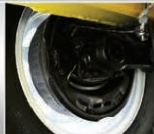
Electric brakes eliminate extra load on vehicle 6438P only
