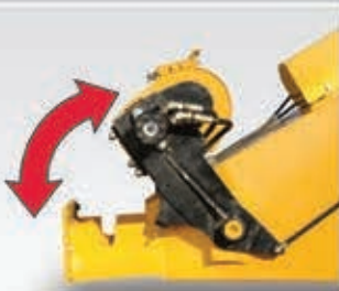
Lift assist for servicing using gas shocks.
