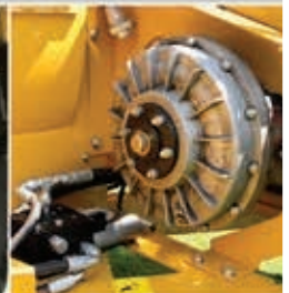
Auto engage fluid coupler is ideal for contractors where heavy duty work is required
