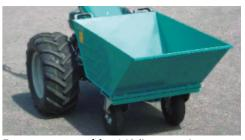
**Front transport bin:** 140 liter capacity, easy to operate tilting device, 2 large pneumatic tires
