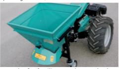
**Spreader for fertilizer, sand or road salt** 100 l, spreading direction adjustable (left-center-right)
