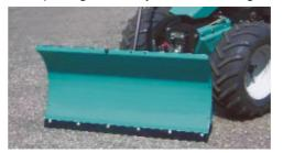
**Front scraper** operating width: 1,000 mm, with spring guard and replaceable scraping slat
