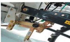
the adjustable depth of the floating plate - to adapt to different fields requirements
