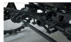
the the lame degree of adaptive swing bracket - easily deal with tilt
