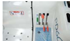
can isolate the arbitrary grouping clutch - the number of rows change
